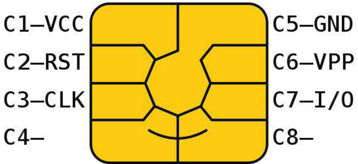
Figure 2.3. Signaling Elements of a Smart Card Chip
