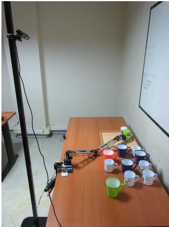
Figure 3.1. Our robot system with 3D depth camera and 5 DOF robot arm.
