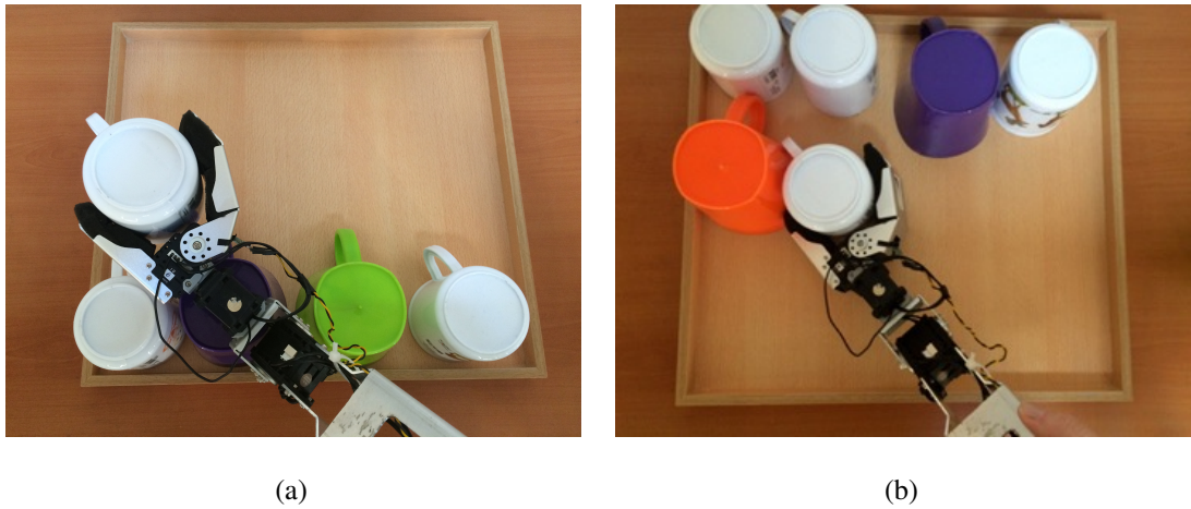
Figure 4.4. (a) Gripper collision with a previously placed mug in the Bottom-Left-Fill approach, (b) No collisions in “Top-Left-Fill” approach.
