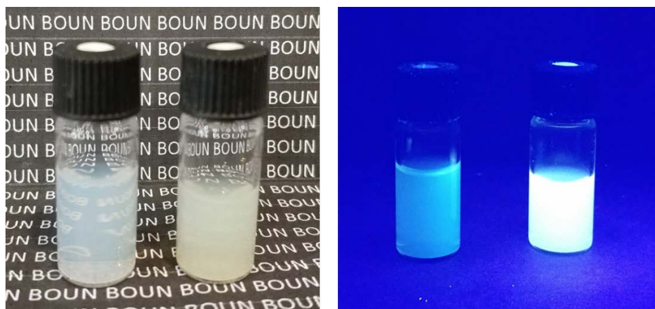
Figure 4. 23. DBM and DTM containing PISA particles under day light (A) and UV irradiation (B).
