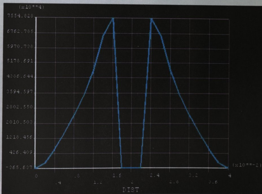
Figure 5.20 Stress distributions (on the inner surface of flanged piece) in terms of SY in the width direction and passing through center of the right spot
