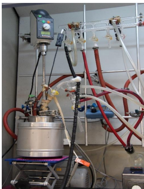
Figure 1.5. Melt polymerization reaction set-up.
