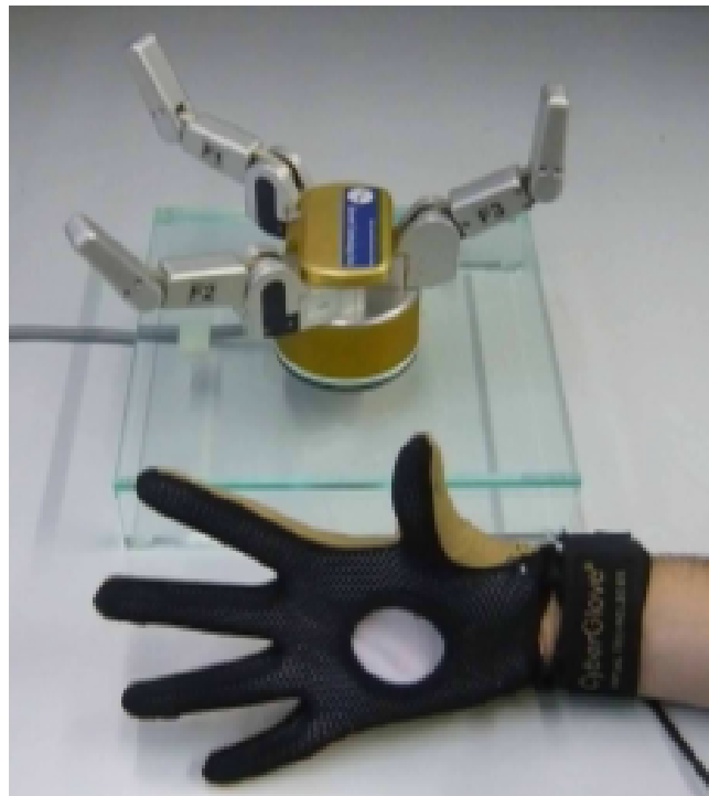
Figure 2.2. A finger type gripper. Reprinted from [21].
