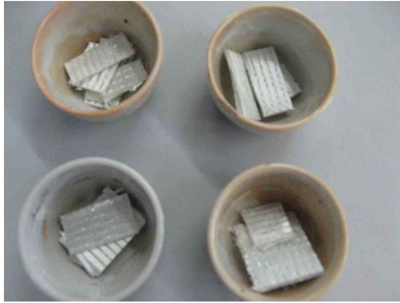
Figure 2.21. Complete burn off of the matrix resulting in only fibers remaining
