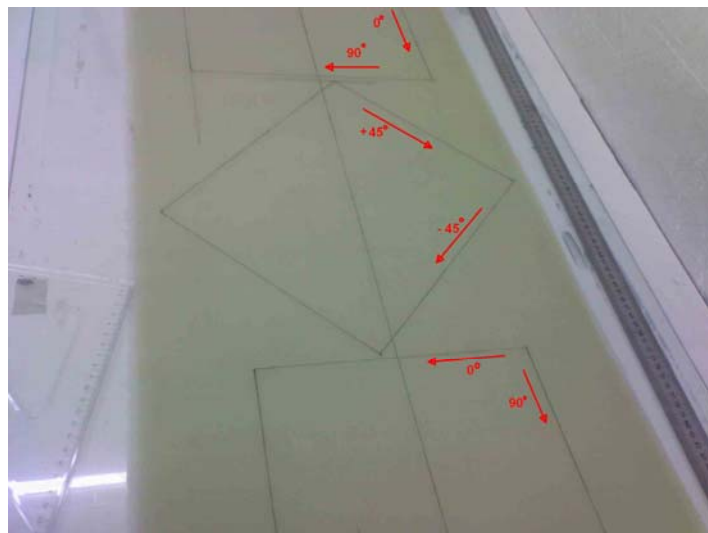
Figure 2.12. Lines are drawn on the material to get desired orientations
