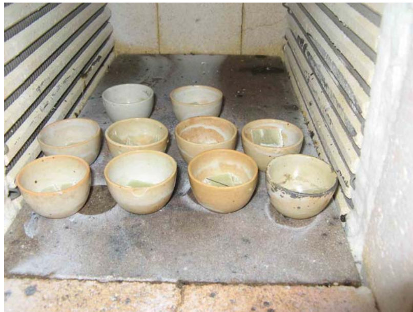
Figure 2.20. Crucibles placed in the muffle furnace
