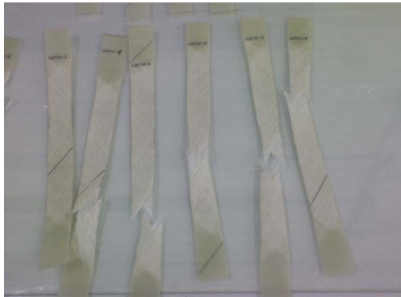
Figure 3.24. Failure of [0/90]_{4s} specimens loaded in 45^\circ direction
