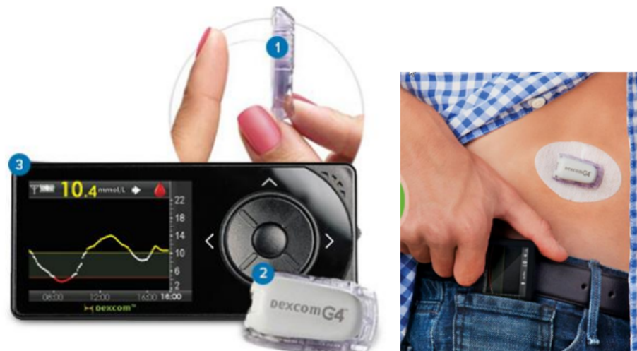
Figure 3.7. Parts of Dexcom or CGM (Sensor, Receiver, and Transmitter) (Dexcom, 2018).
