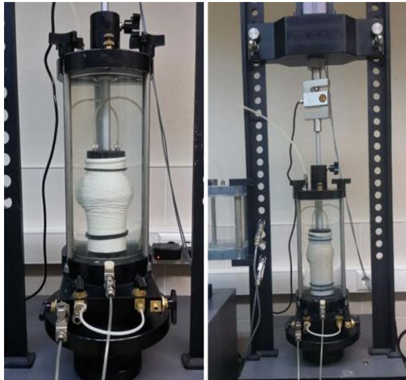
Figure 3.9. Triaxial tests under K_0 conditions.
