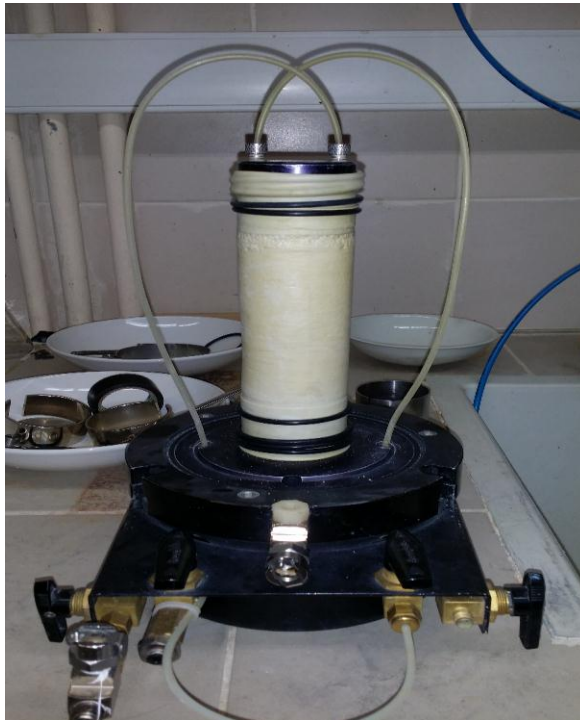
Figure 3.11. View of the test specimen held stable by vacuum pump.
