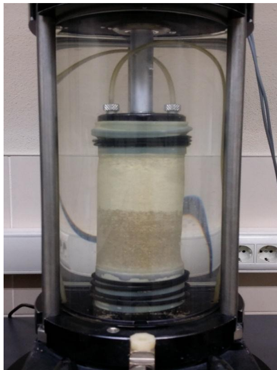
Figure 3.12. Overview of triaxial sample during saturation phase.
