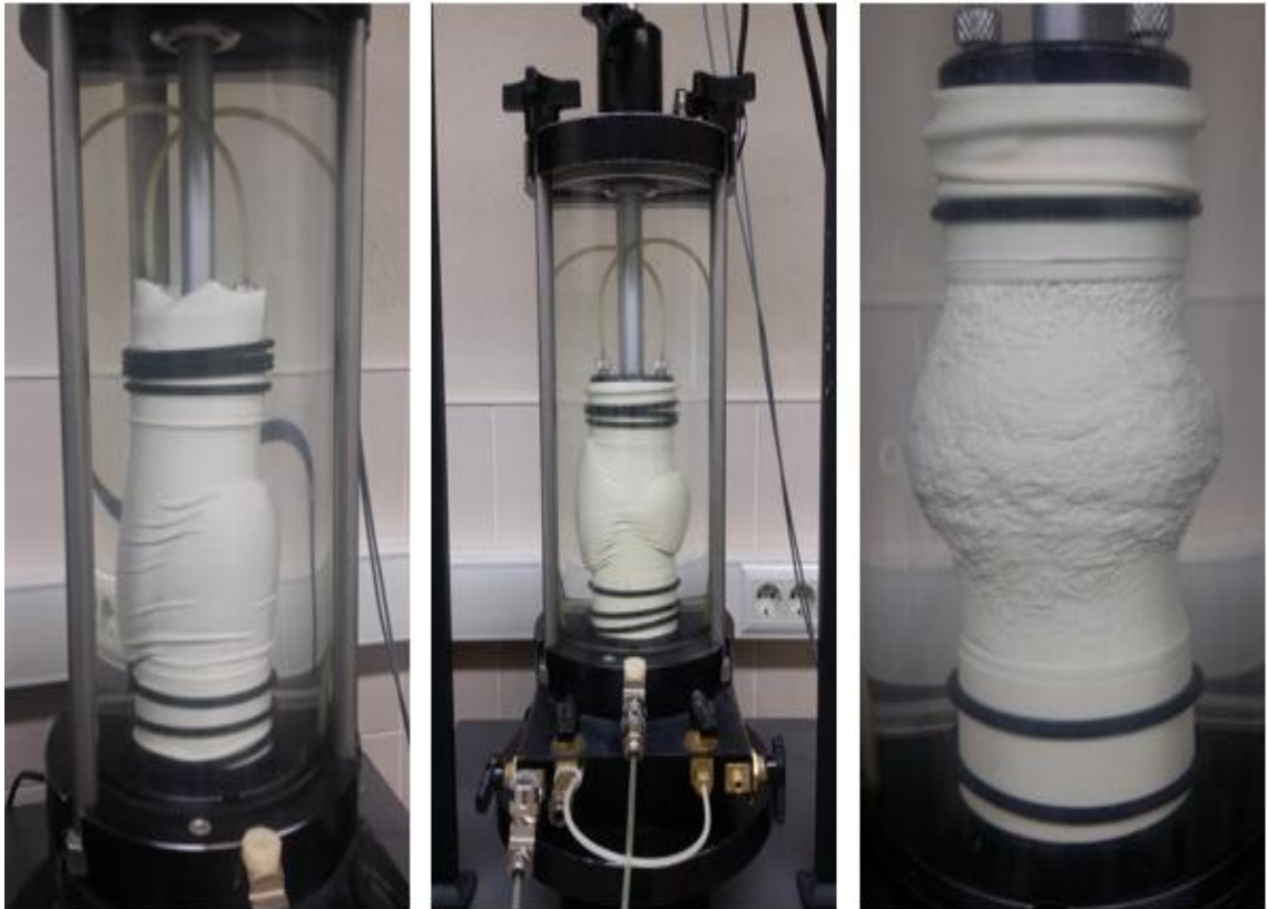
Figure 3.13. View of failed samples after shearing phase.
