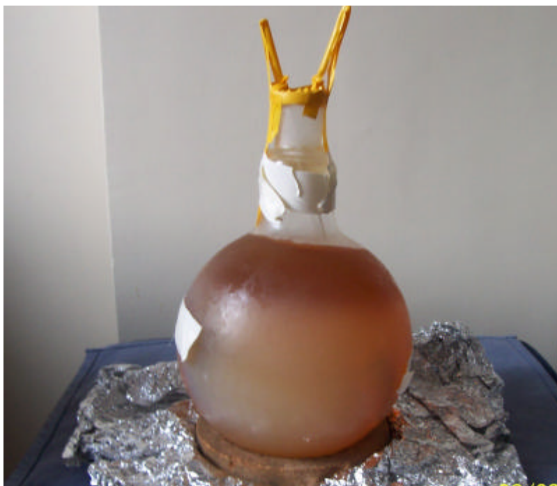
Figure 6.4: The irradiated homogeneous phantom
