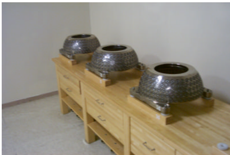
Figure 2.6: The collimator helmets of the Gamma Knife
