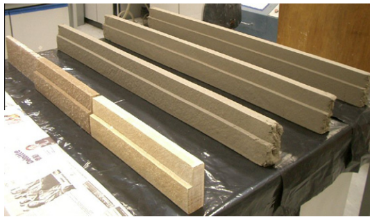
Fig. 3. Extruded door frames (note: in the right three door frames, MOC was partially replaced by fly ash, resulting in dark color, which are products developed in parallel research and beyond the scope of this specific paper).
