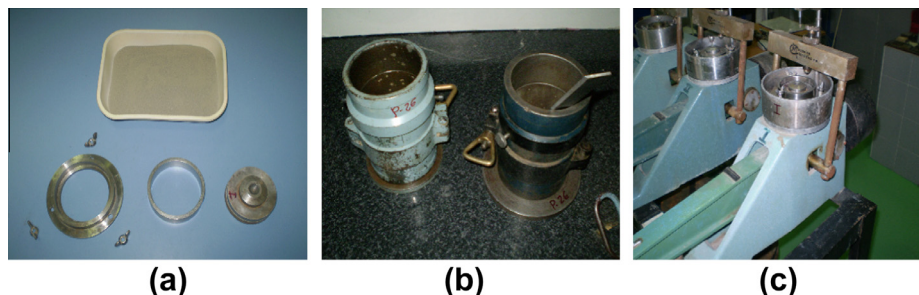
Fig. 2. Pictures of lab equipment: (a) preparation of swelling pressure cell; (b) molds for standard Proctor test; (c) oedometers.
