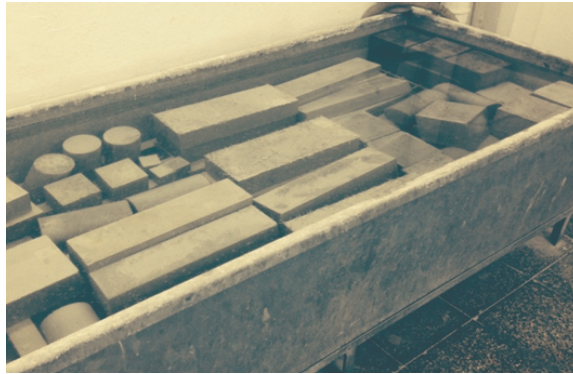
Figure 3.3. Curing of the Specimens in Water Tank.
