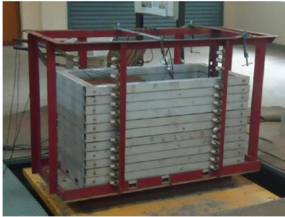
Figure 6.5. Laminar box used for the experiments (Srilatha et al. , 2012).
