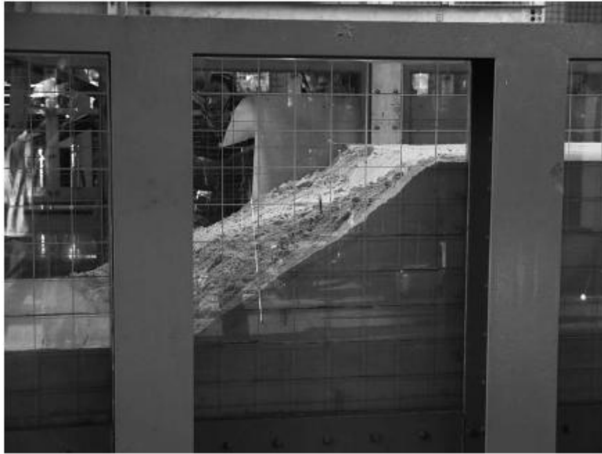
Figure 6.4. Failed slope model after seismic loading (Lin and Wang, 2006).
