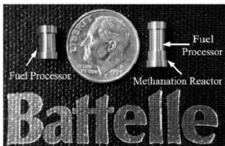
Figure 5.7. Second generation high efficiency micro-scale fuel processor, original (left) and with CO removal reactor (right) (Holladay et al. , 2004b)
