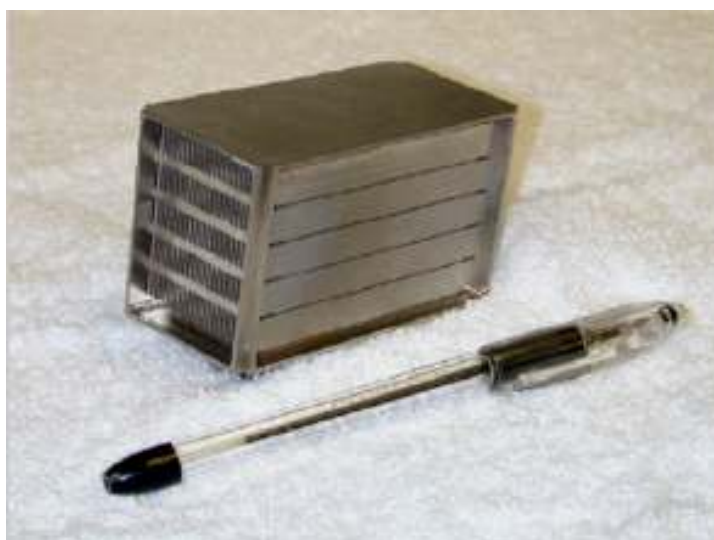
Figure 5.12. Micro-scale differential temperature water-gas shift reactor (Qi et al. , 2007)
