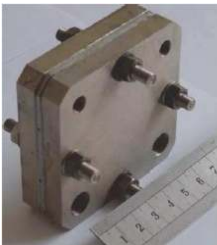
Figure 5.13. Microchannel preferential oxidation reactor (Chen et al. 2004)
