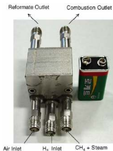
Figure 5.9. Photograph of assembled catalytic combustor/reformer (Ryi et al. , 2005).
