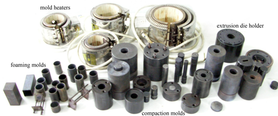
Figure 3.4. The equipment used for PCM foam manufacturing: from left to right; foaming molds, mold heaters, compaction molds, extrusion die and die holder
