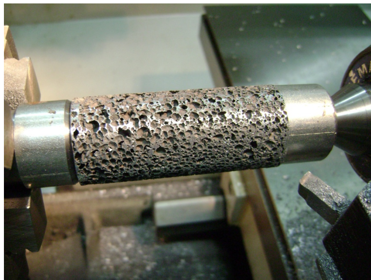
Figure 3.7. Removal of the outer solid skin of foams by machining
