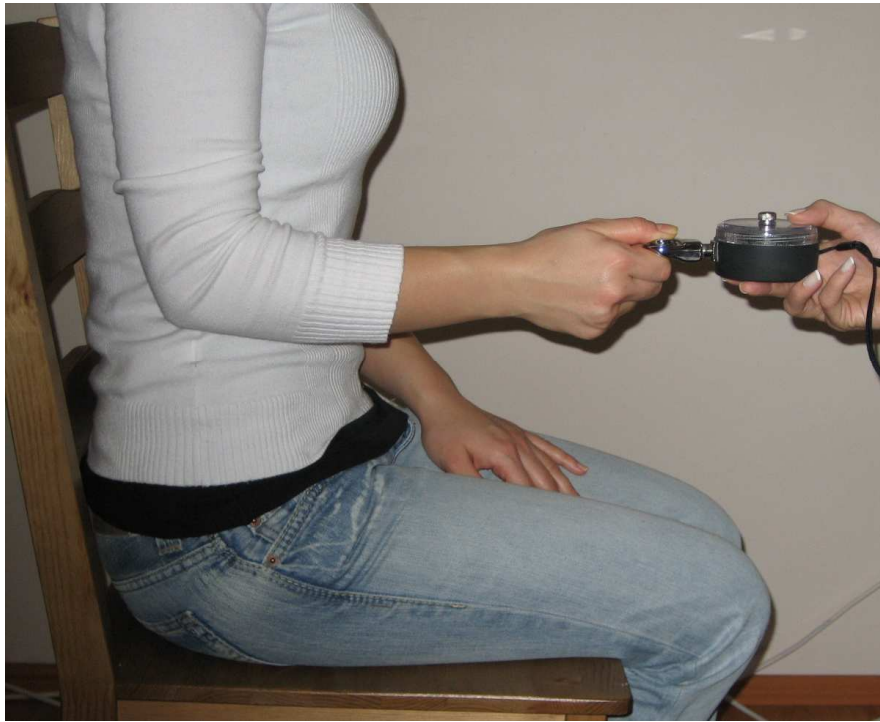
Figure 4.8. Measurement of lateral pinch strength while sitting
