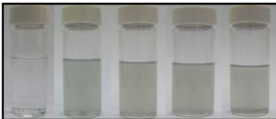
Figure 5.8. Dispersion of BNNTs in acetone solution after 0, 15, 30, 45 and 60 minutes of high power ultrasonication, respectively
