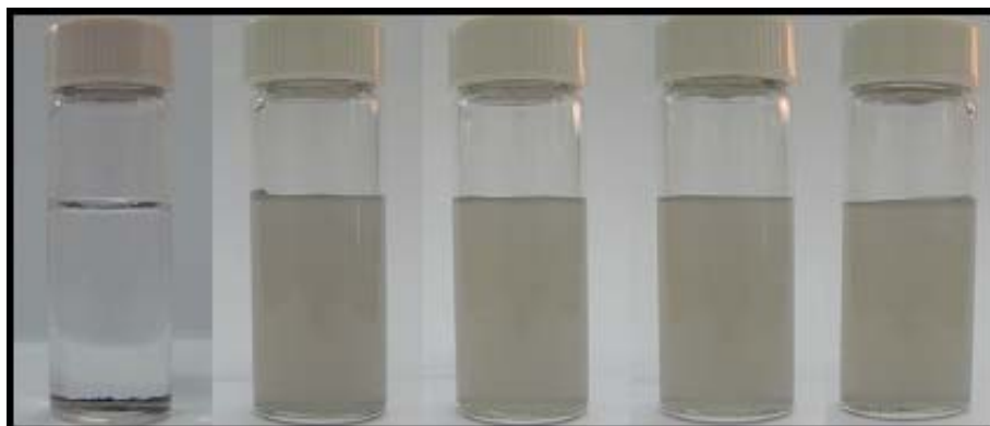
Figure 5.10. Dispersion of BNNTs in DMF solution after 0, 15, 30, 45 and 60 minutes of high power ultrasonication, respectively
