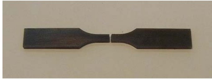
Figure 5.14. Typical broken tensile test specimen
