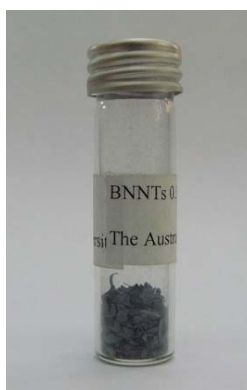
Figure 4.1. 250 mg as-received BNNT (The diameter of the bottle is 15 mm)
