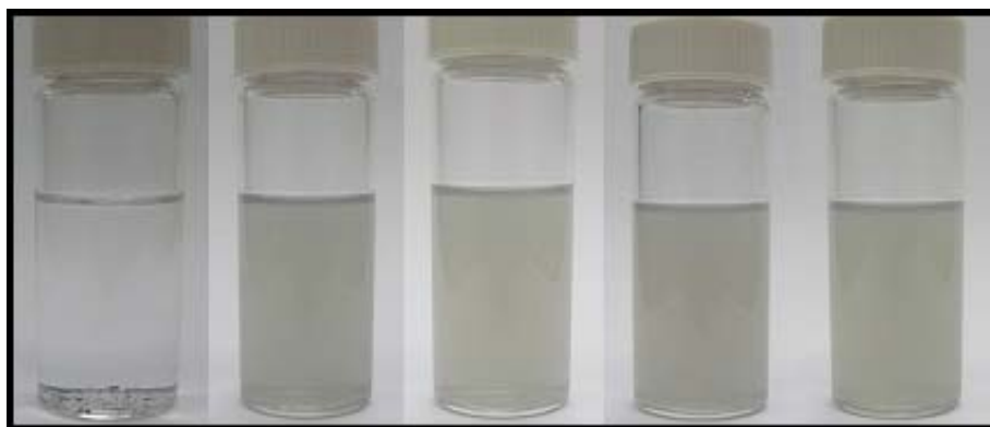
Figure 5.9. Dispersion of BNNTs in ethanol solution after 0, 15, 30, 45 and 60 minutes of high power ultrasonication, respectively
