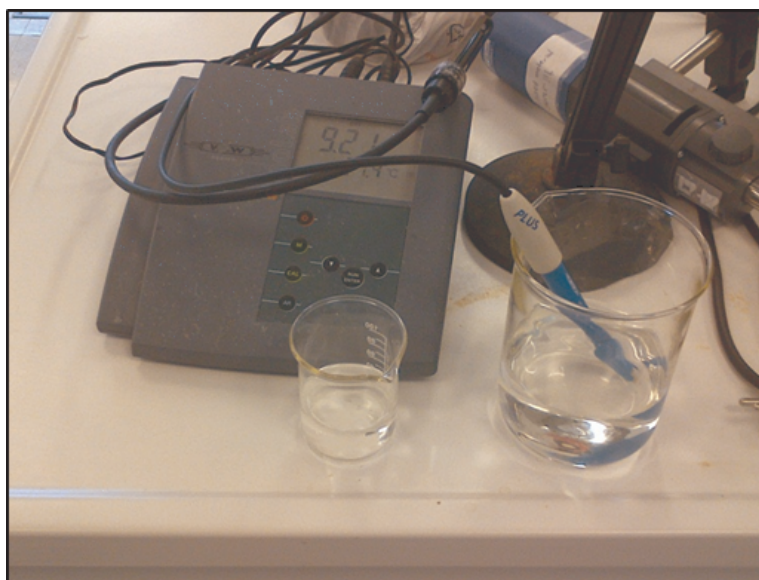
Figure 4.11. Measuring of pH of magnetically treated water.
