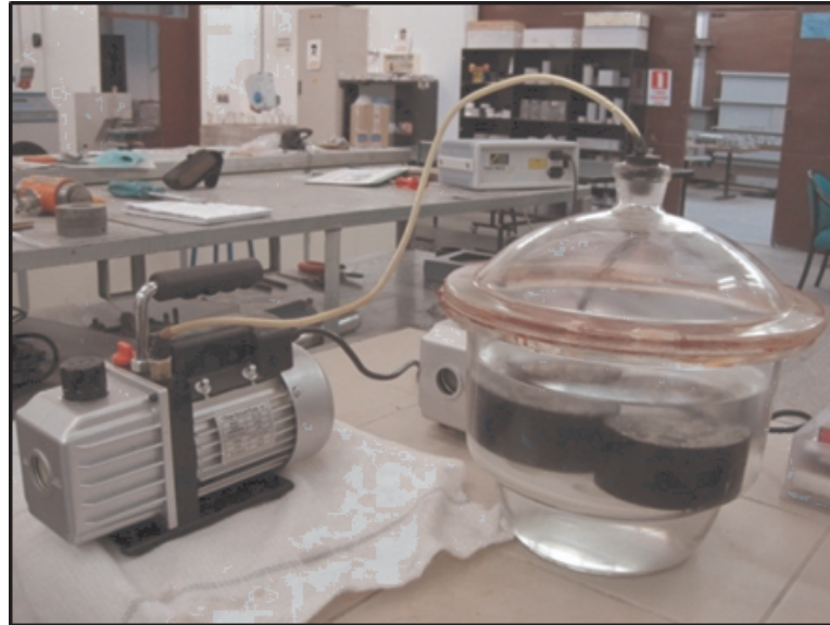
Figure 4.15. Soaking of concrete specimen in the desiccator.
