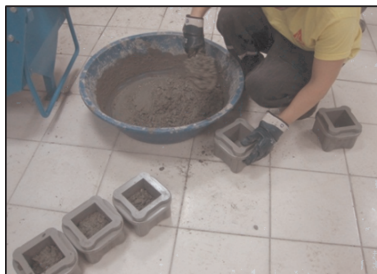
Figure 3.2. Casting of concrete in molds.
