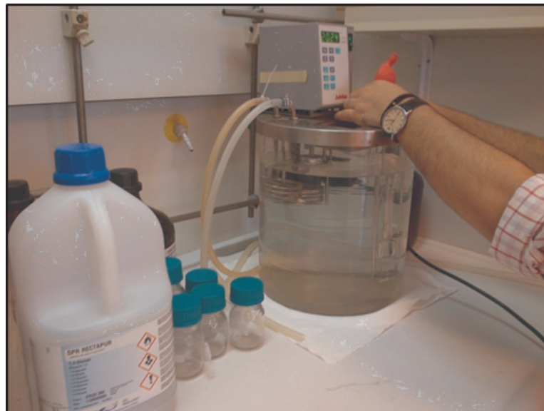
Figure 4.10. Suction of water in the viscometer.
