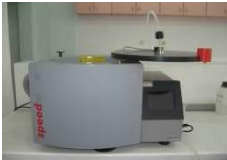
Figure 3.2 The microwave system used in the study (Berghof Speedway MWS+3).
