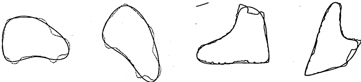
Figure 3.2: Implicit polynomial fittings to car and hikingboot, and one of their affine transformations. Small dots are the data sets, darker lines are the zero set of the best fit 4th degree IP models.
