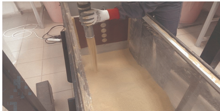
Figure 3.11. Placement of the Sand by Pluviation Method.
