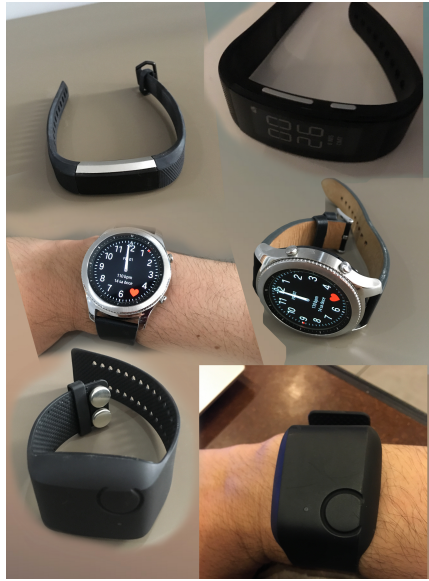
Figure 3.1: Wearable Devices for collecting data in Daily Life (Left Top: Fitbit, Right Top: Sony Smartband, Middle: Samsung Galaxy Gear S3, Bottom: Empatica E4)
