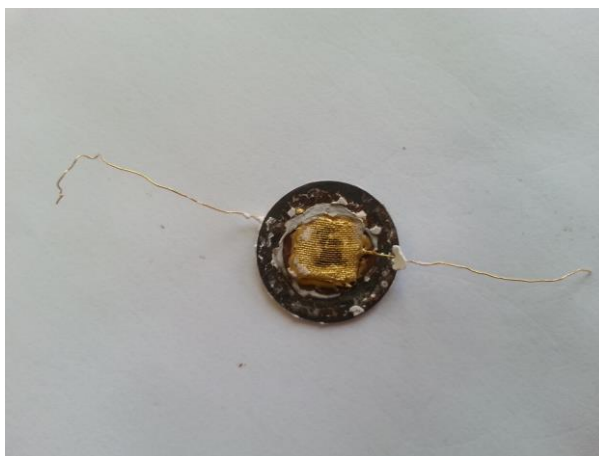
Figure 2.4. Mn impregnated disc anode side taken out of the test tube.
