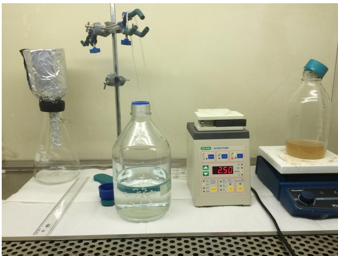
Figure 4.2: Ca-alginate bead preparation setup
