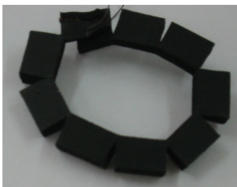
Figure 3.3. The image showing the circular strip geometry of PU/PPY foam used during pyrrole formation
