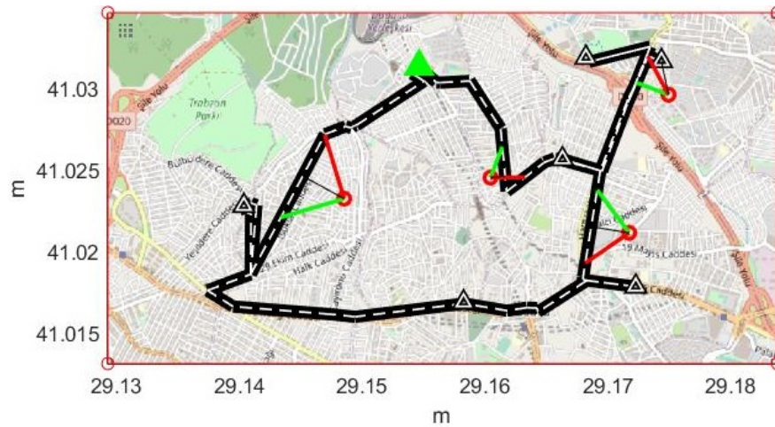
Figure 2.1. Simultaneous Resource-aware Cooperative Delivery Mission of an AGV and a UAV.
