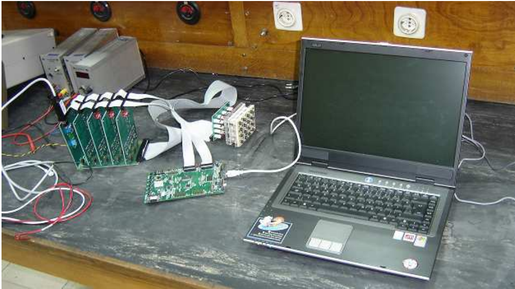
Figure 3.15 Instrumentation that includes microphone array, instrumentation amplifiers, filters, ADC's, Cypress EZ-USB FX2 developer kit and PC
