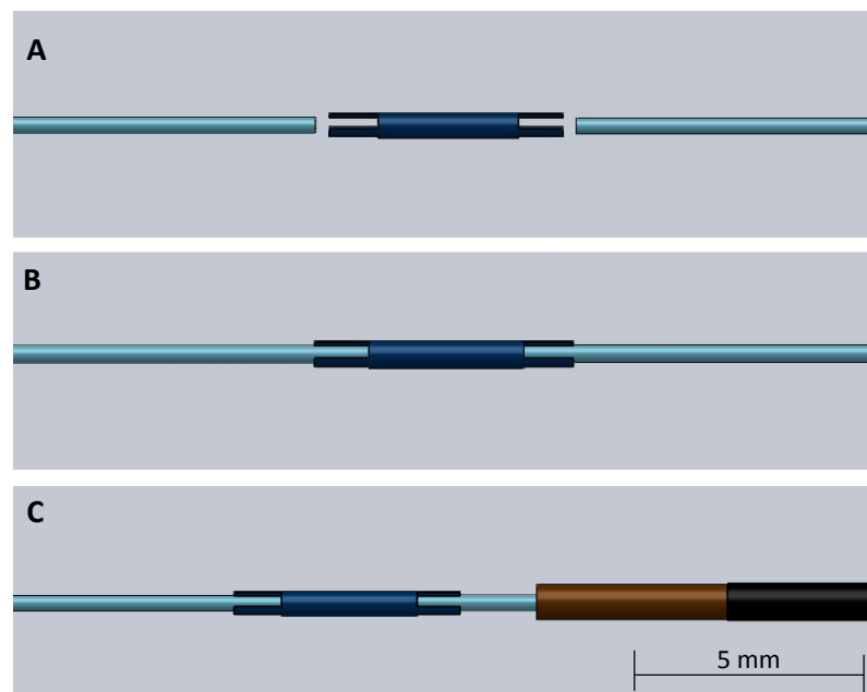
Figure 2.1 The core of the MR-safe segmented guidewire is constructed using insulated 10-cm rod segments and connectors (A), which are interconnected (B) to form a full-length core structure. A 260-cm prototype consists of 25 such connections; which is then jacketed with a polymer-braided tube, and an outer-most layer of thermoplastic polymer is melted over the braided jacketing to complete the device (C).
