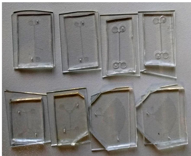
Figure 5.15. Four pairs of microchannels obtained for experiments. Top left right pair was to used in the subsequently presented results since it lets through a higher sample volume.
