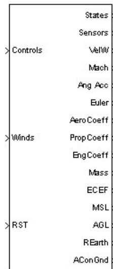
Figure 2.2. 6-Dof Aircraft Model Block
