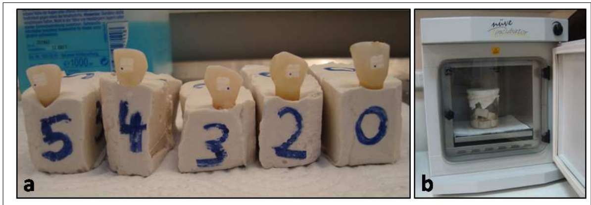
Figure 3.7 (a) A group of teeth after bonding procedure, (b) Groups, inside a beaker, were kept in an incubator for 2 days.
