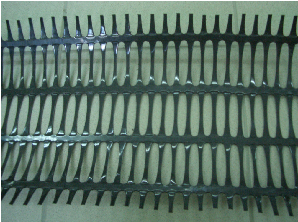
Figure 3.5. Picture of Geogrid II (uniaxial geogrid) used in connection tests
