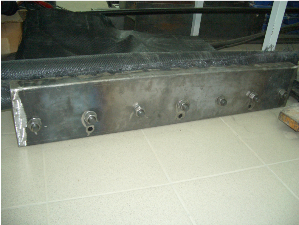
Figure A.2. The clamp and the three holes on the clamp
