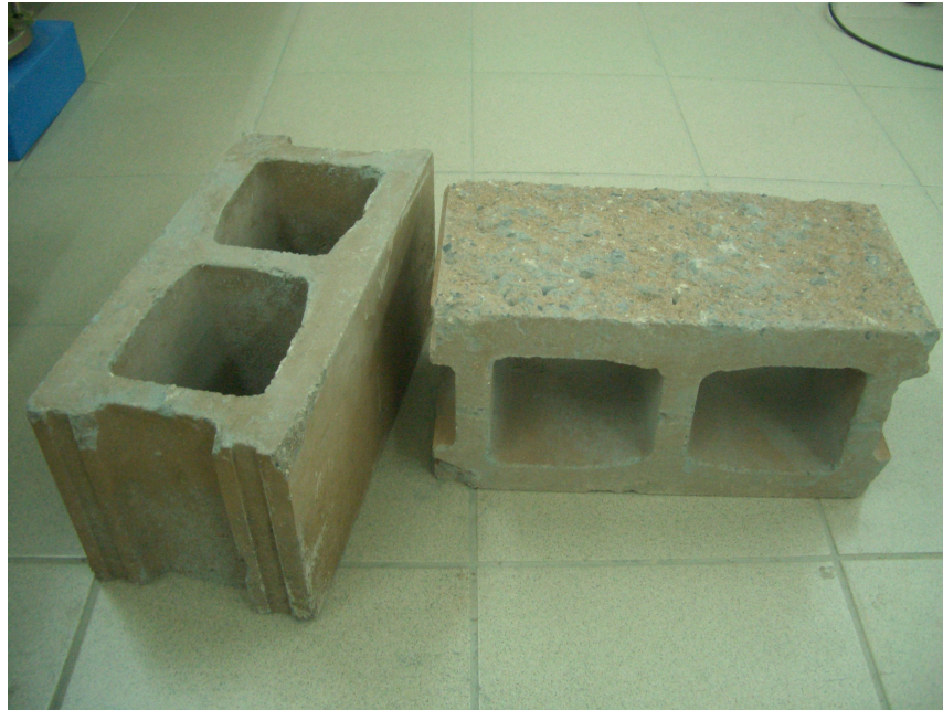
Figure 3.1. Picture of concrete blocks (Tech Block) used in connection tests
