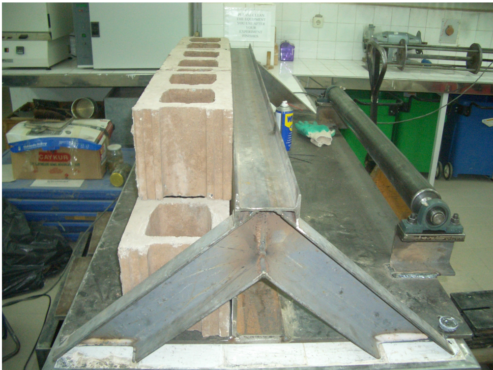
Figure A.3. Picture of the test apparatus and precast concrete block facing elements
