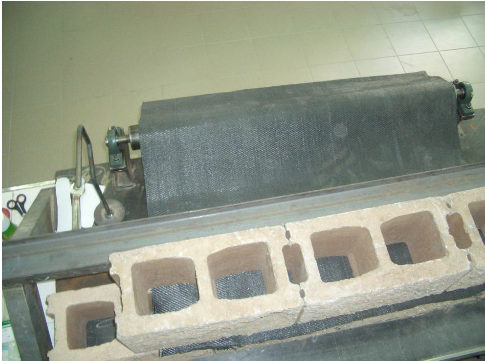
Figure A.4. The top view of the test apparatus and precast concrete block facing elements
