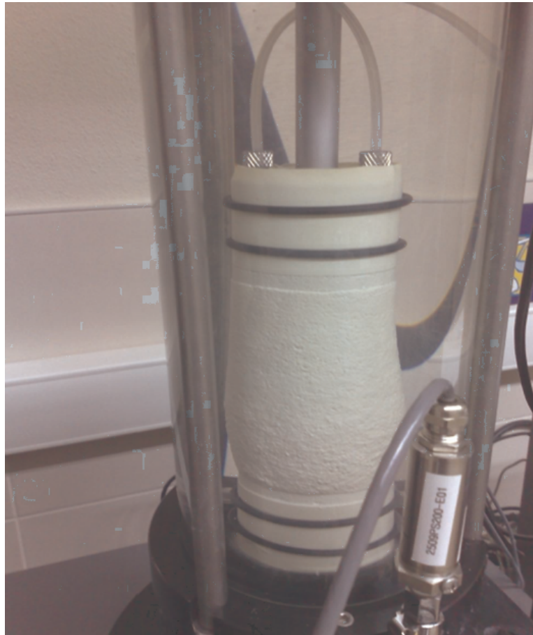
Figure 3.14. Parabolic Shape of the Sample During Shearing (Abadkon, 2012).
