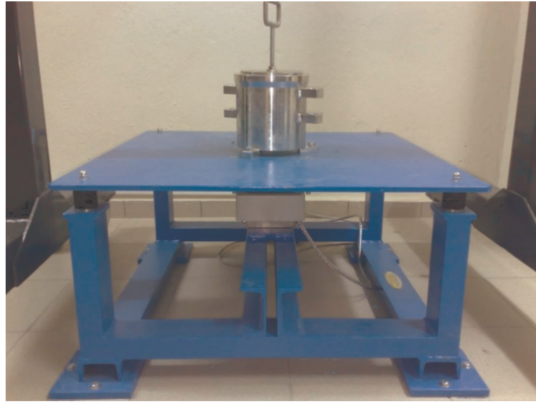
Figure 3.2. Vibratory Table Used to Determine Maximum Minimum Void Ratios.
