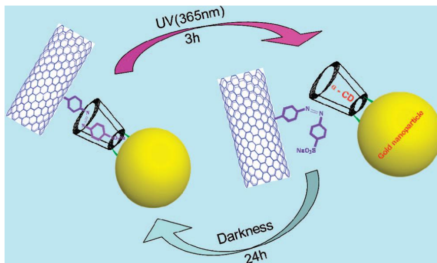
Figure 1.7. Schematic presentation of gold nanoparticles' reversible attachment onto and detachment from the surface of MWNTs through the photochemically controlled host-guest molecular recognition interaction.
