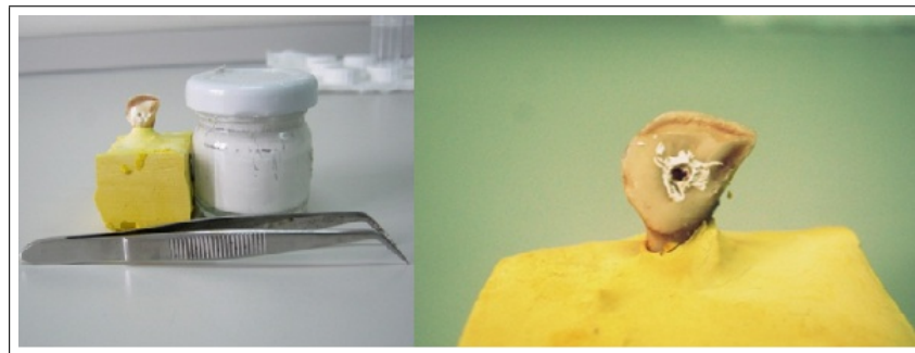
Figure 3.11 Silicon Thermal Paste to Mimic The Tissue.
