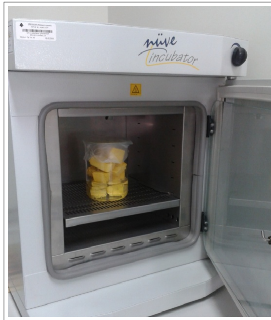
Figure 3.6 Samples are kept in the incubator for the composite polymerization.
