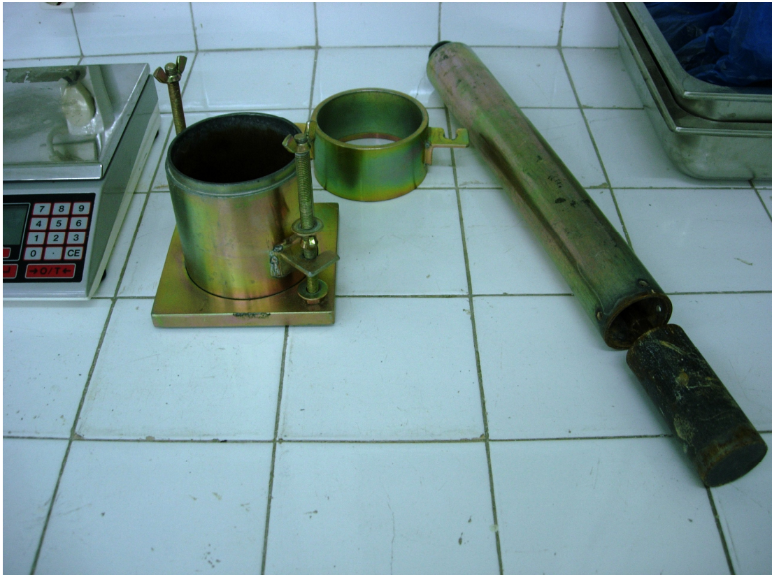
Figure 4.8. Compaction mold and hammer
