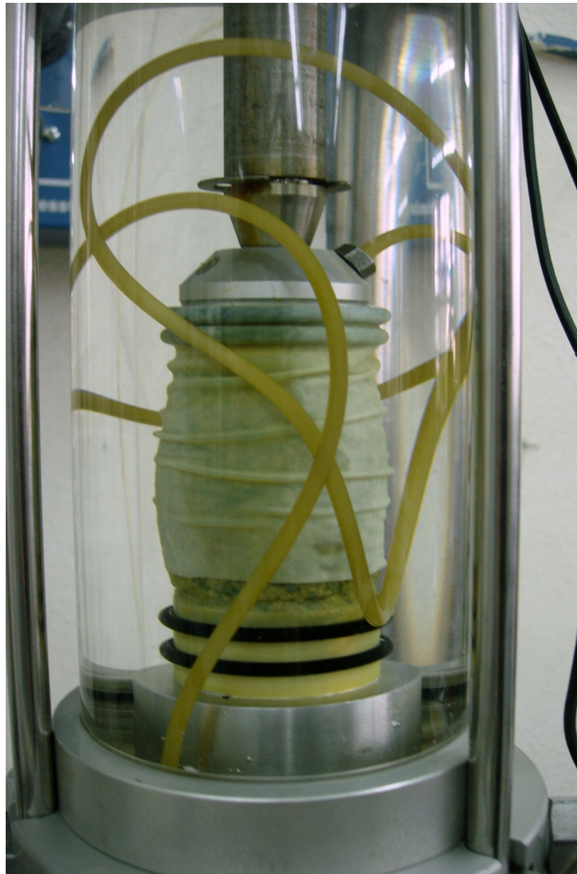
Figure 4.21. Example of a failed specimen
