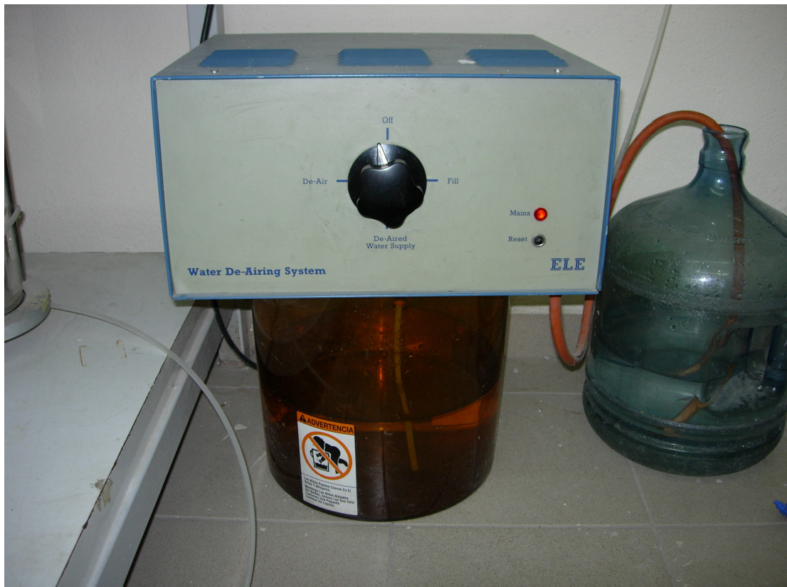
Figure 4.20. De-aired water supply
