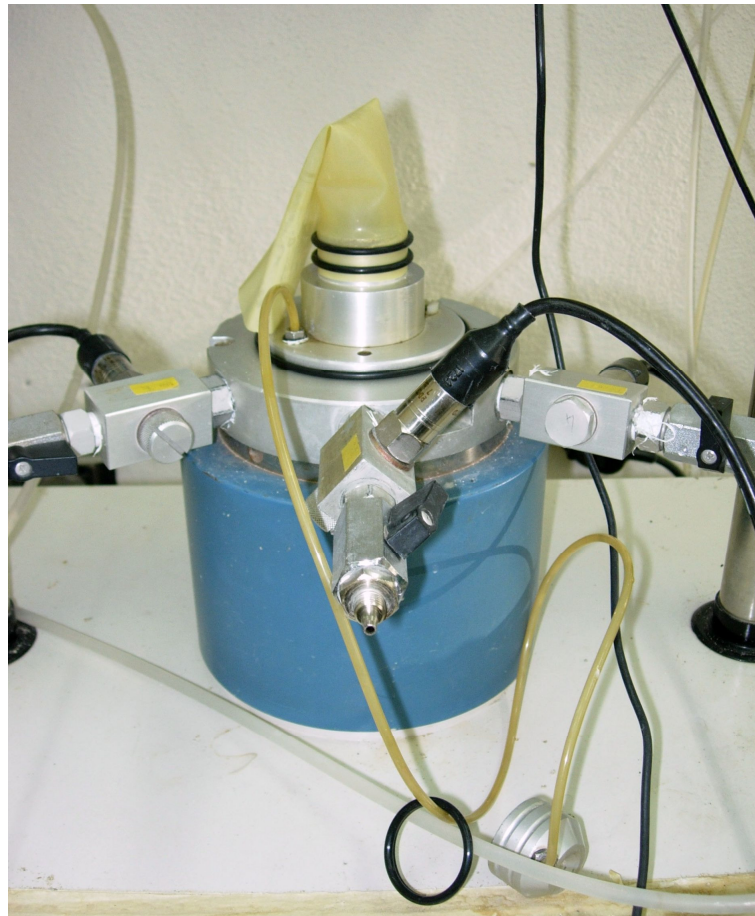
Figure 4.13. Rubber membrane attached to the base platen using “O” rings
