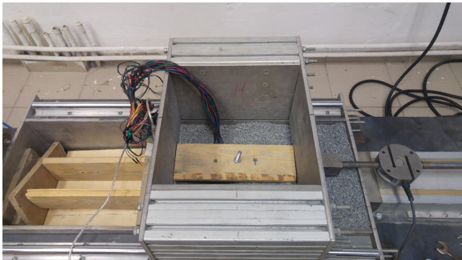
Figure 3.11. The pile in the test box.
