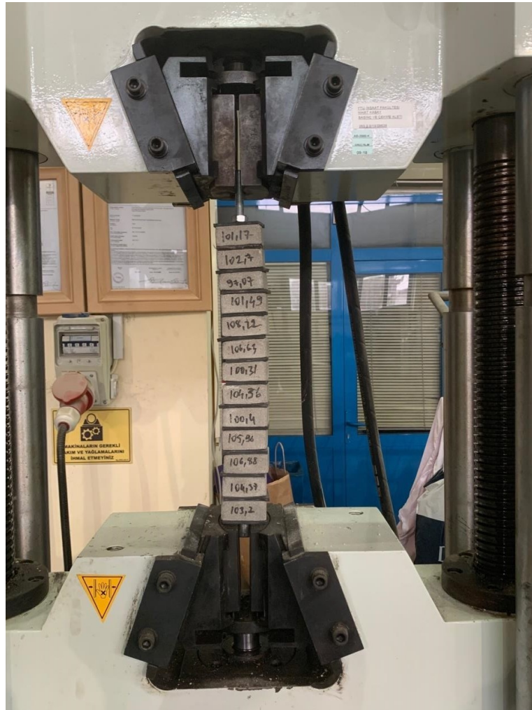
Figure 3.3. Steel tension test device.
