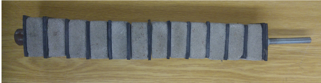
Figure 3.2. Model pile after assembling.
