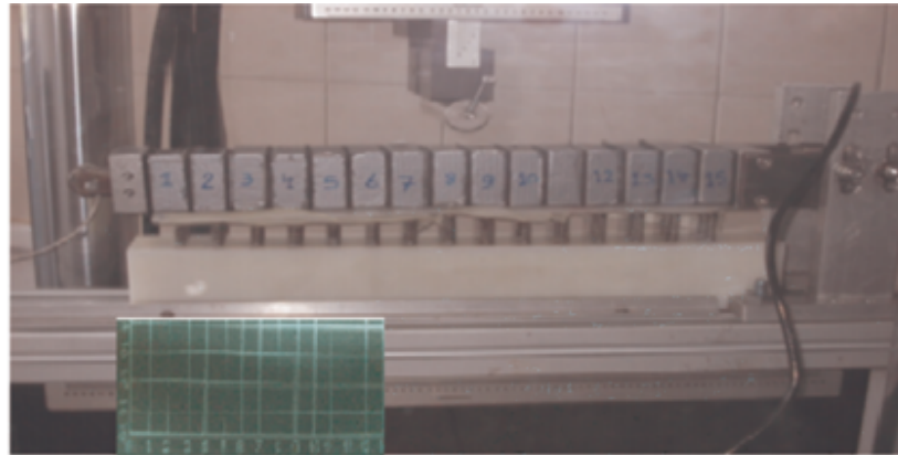
Figure 2.12. Segmental pile with variable flexural rigidity [11].
