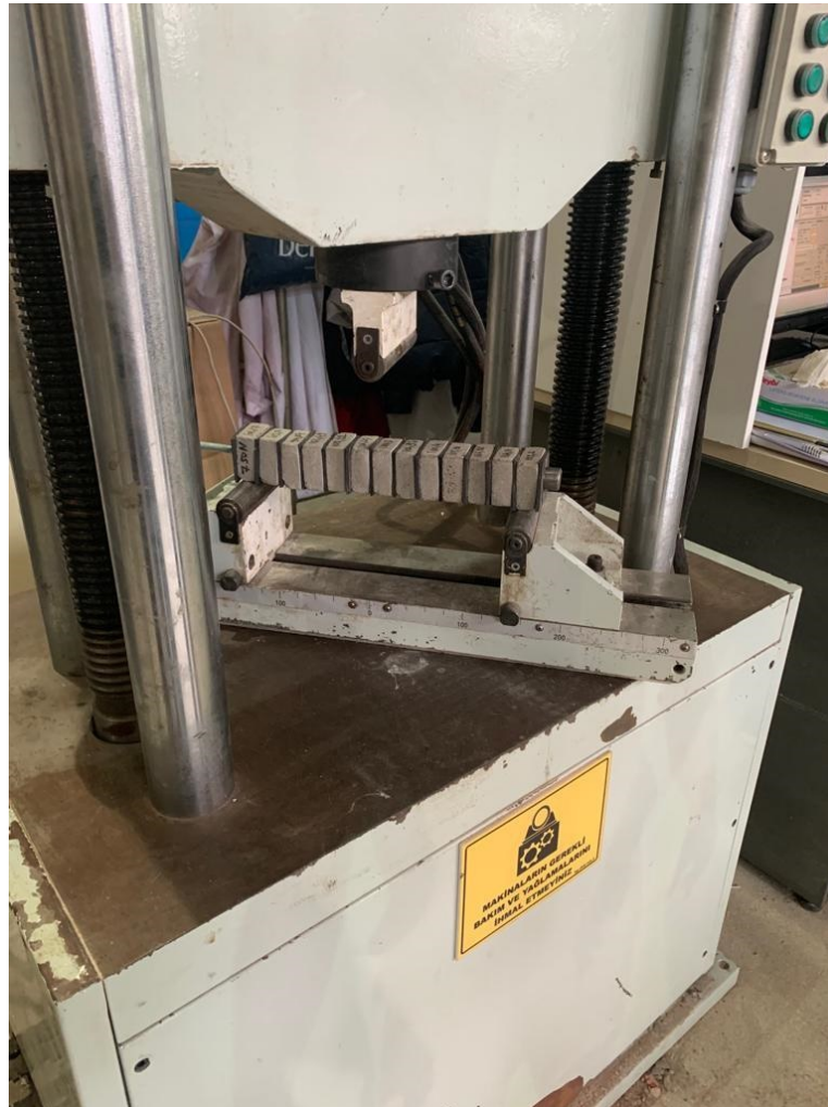
Figure 3.4. Three point bending test device.
