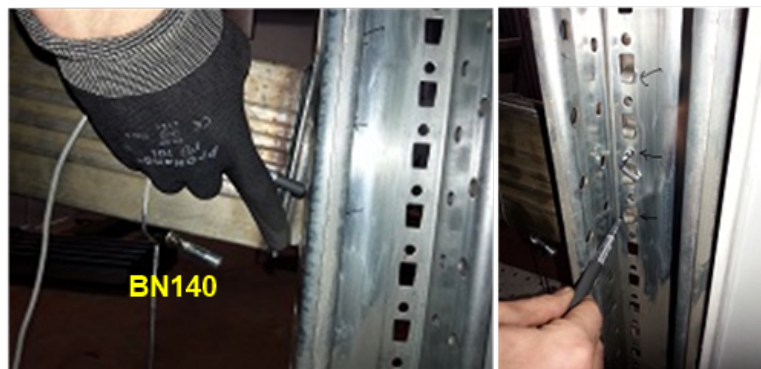
Figure 3.18. Failure Modes in Monotonic Tests on BN140 Specimens.
