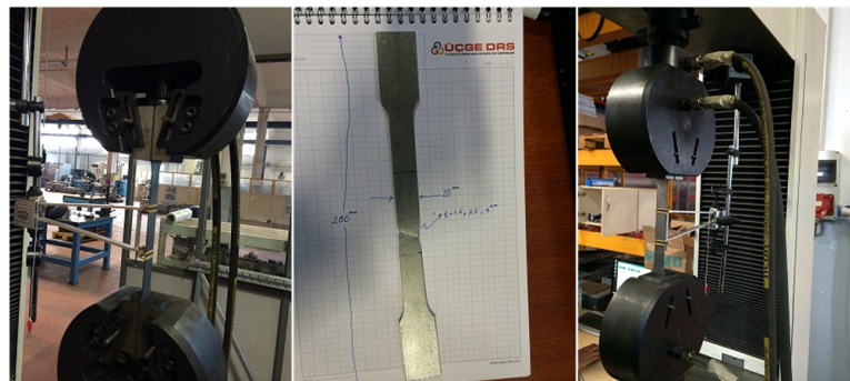
Figure 2.16. Coupon Test for Obtaining Yield Value of Material.
