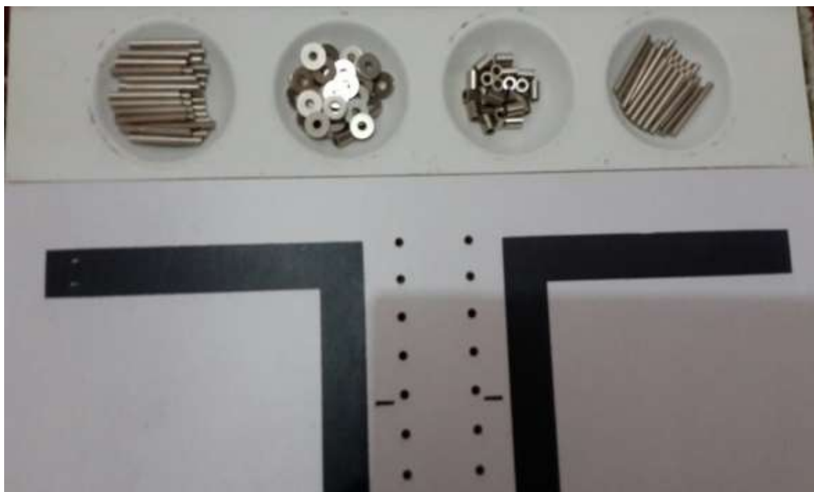
Figure 4.8. Pins (from left in first and fourth cup), washers (in second cup) and collars (in third cup).
