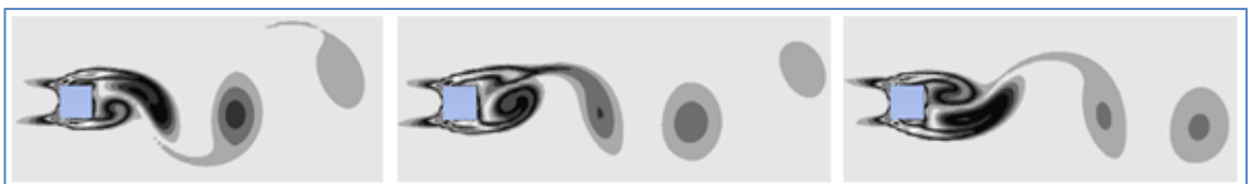
Figure 4.22. Square cylinder Wake region vorticity profile, Newtonian Fluid ( Re = 500 ).
