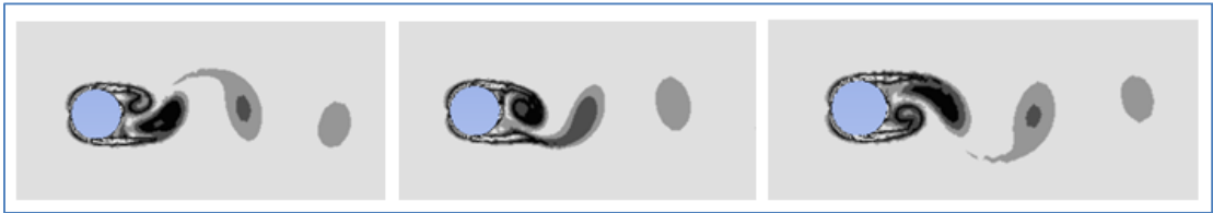
Figure 4.8. Circular cylinder wake region vorticity profile, Newtonian fluid ( Re = 200 ).
