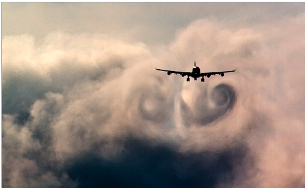
Figure 1.3. An example of turbulent flow in an airplane wake region [37].
