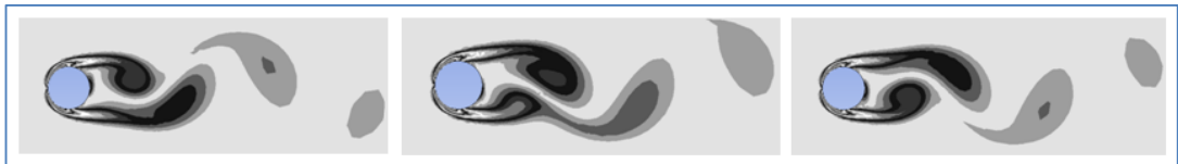
Figure 4.15. Circular cylinder wake region vorticity profile, Power-law fluid (80 wppm, Re = 200 ).
