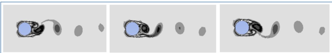
Figure 4.11. Circular cylinder wake region vorticity profile, Newtonian fluid ( Re = 2000 ).
