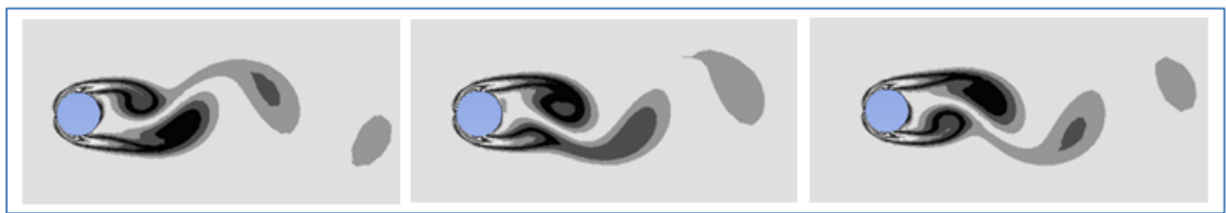
Figure 4.10. Circular cylinder wake region vorticity profile, Newtonian fluid ( Re = 1000 ).
