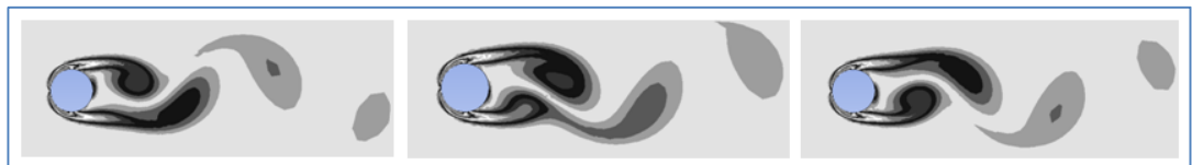
Figure 4.16. Circular cylinder wake region vorticity profile, viscoelastic FENE-P model ( We = 0.05 , L = 30 , Re = 200 ).
