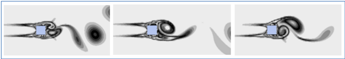
Figure 4.25. Square cylinder wake region vorticity profile, Power-law fluid model, 40 wppm ( Re = 1000 ).
