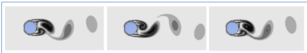
Figure 4.18. Circular cylinder wake region vorticity profile, viscoelastic FENE-P model ( We = 0.05, L = 30, Re = 500 ).
