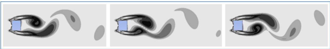
Figure 4.21. Square cylinder wake region vorticity profile, Newtonian Fluid ( Re = 200 ).
