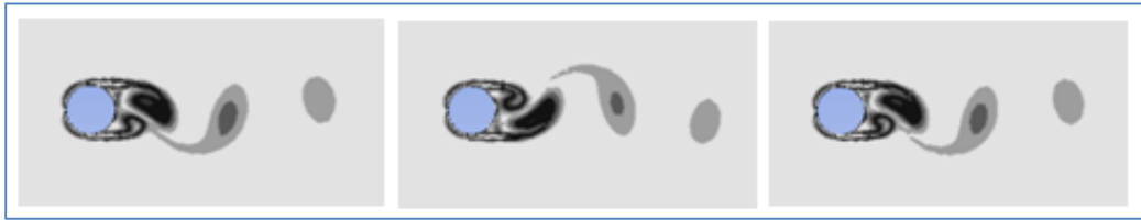
Figure 4.17. Circular cylinder wake region vorticity profile, Power-law fluid (80 wppm, Re = 500 ).
