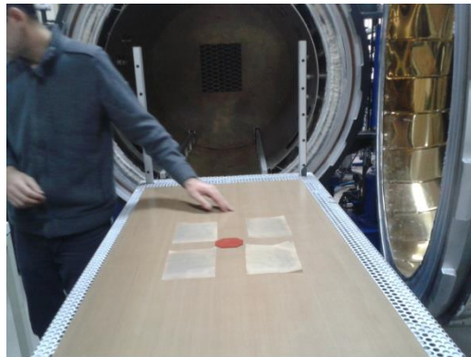
Figure 3. 3. Placement of the stacked plates the specimens on the table with a Teflon cover.
