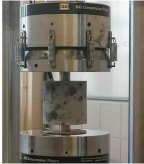
Figure 3.7. Double-punch test frame.
