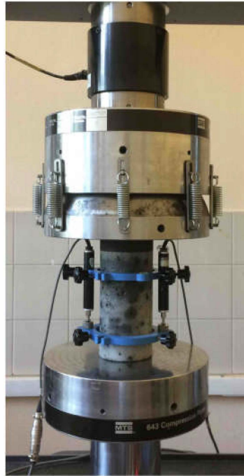
Figure 3.4. Modulus of elasticity test frame.
