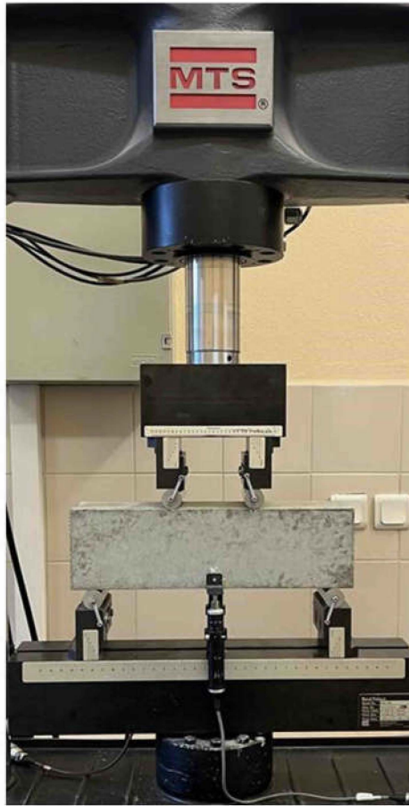
Figure 3.5. Plain concrete bending test frame.
