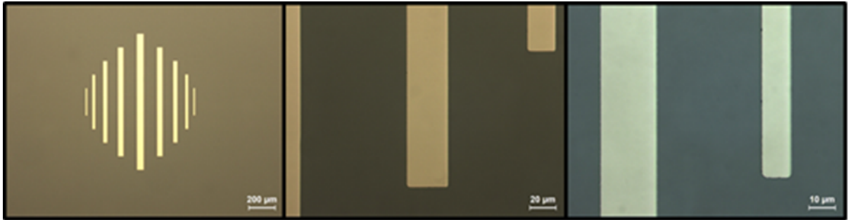
Figure 4.1. Sputtering rate measurement procedure. From left to right, one single calibration grating, and partial images of gratings to be measured.
