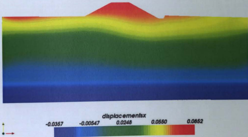
Figure 8 - 6: Horizontal displacements under seismic excitation at t = 40 seconds on the deformed shape of the structure. (meter).
