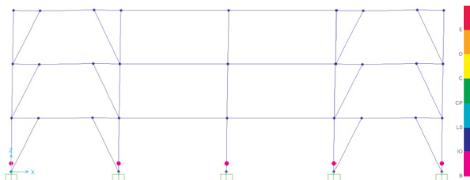
Figure A.7. Formation of the Plastic Hinge for Mid Rise EBF with Short Link Using BRBs.
