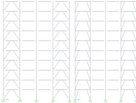
Figure 7.5. Eccentric Braced Frame in the Long Link (Left) and Short Link (Right) Shape.
