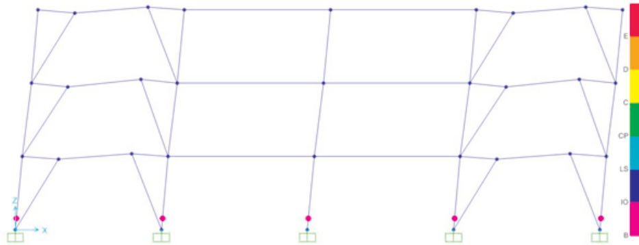
Figure 8.19. Formation of Plastic Hinge for EBF with Long Link Using BRBs (SAP 2000).
