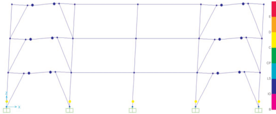
Figure A.8. Plastic Mechanism for Mid Rise EBF with Short Link Using BRBs.
