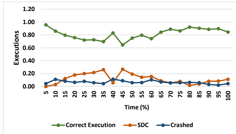
Figure 4.23. Correlation of fault injection timing with the Susan smoothing application execution.
