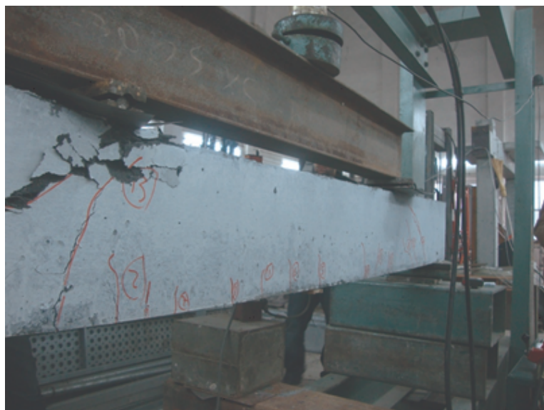
Figure 4.20. Crack propagation of B-07.
