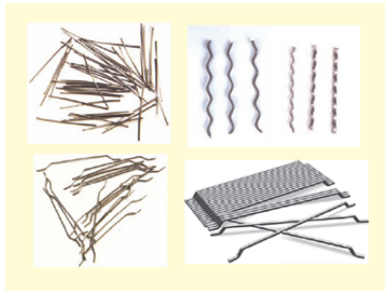
Figure 2.7. Various types of steel fibres (Yerlikaya, 2005).
