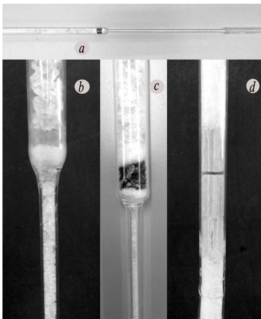
Figure 3.9. Quartz tube reactor filled with quartz chips (a) Whole reactor, (b) Particulate catalyst, (c) Particulate catalyst (crushed monolithic particulate) and (d) Cordierite monoliths.
