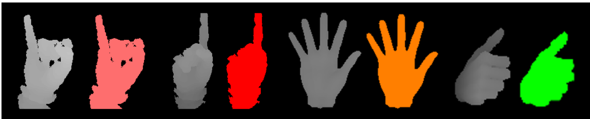
Figure 4.3. Sample RDF-S training images: The first four images are real depth images and their labels, and the rest of the images are synthetic depth images and their labels.
